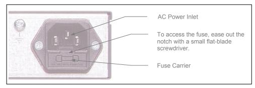
Figure 7.2 Fuse Carrier
